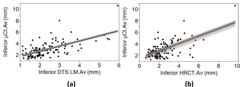
**Fig. 3.** Mixed regression plots of (a) inferior DTS.LM.Av vs.  $\mu$ CT.Av,  $R^2_{Adj} = 0.47$  and (b) inferior HRCT.Av vs.  $\mu$ CT.Av,  $R^2_{Adj} = 0.51$ . The closeness of individual regression lines indicates that the effect of donor on the regression equation is small.
