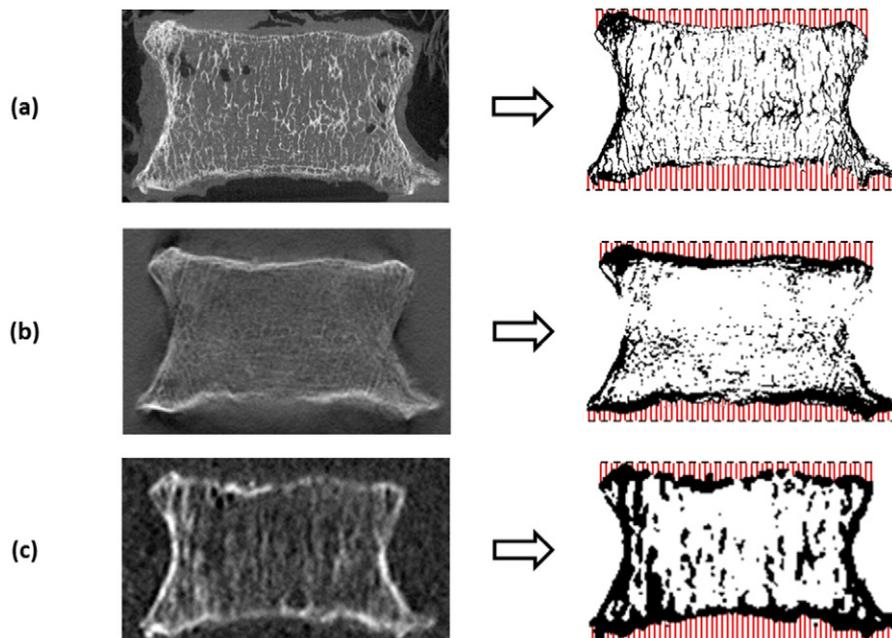
**Fig. 1.** Images were thresholded and depth distributions calculated from a fixed plane (dashed lines) at the superior and inferior endplates. Comparison of images taken from sagittal plane in similar regions from (a)  $\mu\text{CT}$ , (b) DTS (AP), and (c) HRCT. Images are resized to show detail at comparable scale.
