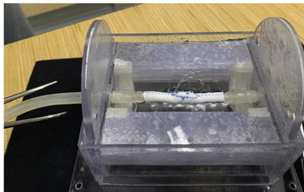
**Fig 3.** The anastomosis vessel segments were attached to a 3D-printed Plexiglas box, which was attached to a bag of saline pressurized at 150 mm Hg, and opened for 5 seconds. In this way, the anastomoses were tested for leaks that were quantified as minor (needle holes) and major (obvious defects), and the total leaked volume was also measured.
