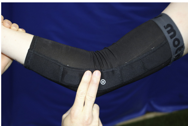
Fig 1. Wearable baseball compression sleeve with a sensor device. Pictured is a wearable baseball compression sleeve on a right elbow, with a sensor device at the medial elbow. The device is placed so that the sensor rests 1.5 inches (approximately 2 fingerbreadths) distal to the medial epicondyle of the humerus, as directed by the device manufacturer's instructions. The medial epicondyle is depicted by the circle on the sleeve.
