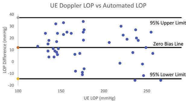
**Fig 2.** Bland–Altman plot of limb occlusion pressure (LOP) difference between proposed technique and manual Doppler technique for the upper extremity (UE). Mean difference is shown (zero bias line) plus or minus 2 standard deviations (95% confidence interval).
