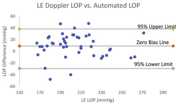
**Fig 4.** Bland–Altman plot of limb occlusion pressure (LOP) difference between proposed technique and manual Doppler technique for the lower extremity (LE). Mean difference is shown (zero bias line) plus or minus two standard deviations (95% confidence interval).
