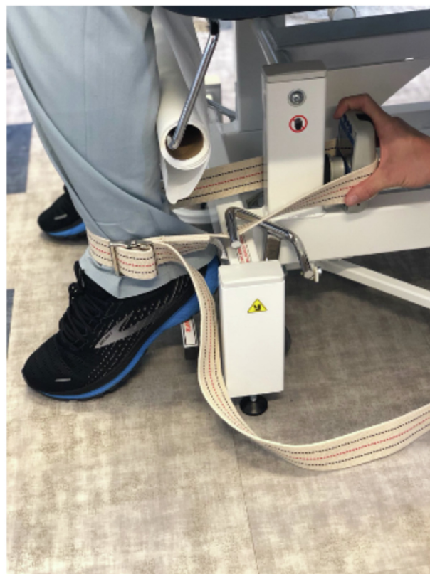
Fig 3. Demonstration of belt stabilized handheld dynamometer placement used to measure quadriceps strength.
